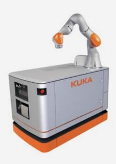
Mobile collaborative robot of medium-large size. Omnidirectional handling system. Manipulator architecture with 7 axes (redundant), ideal for complex kinematics tasks. Equipped with Schunk collaborative electric gripper.
