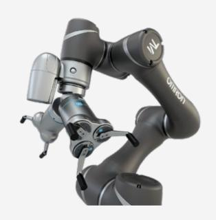
Collaborative robot that has already integrated a vision system that enables visual power assistance, inspection and measurement. Its ability to be integrated with mobile robots allows completely autonomous applications of machine tending and logistics management.
