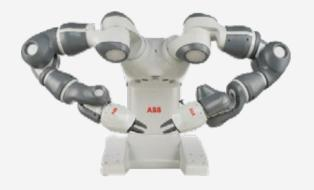
Small collaborative robot. Dual-arm architecture with 7 axes per arm (redundant), ideal for complex kinematic tasks. Equipped with electric gripper and suction cup (arm 1) and electric gripper and camera (arm 2).
