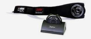
Zephyr BioHarness 3 is a chest strap made of conductive tissue (Smart Fabric patented) within which it is integrated a multi-parameter wearable sensor capable of simultaneously measuring: heart rate, ECG, respiratory rate, body temperature, activity, acceleration and posture.
