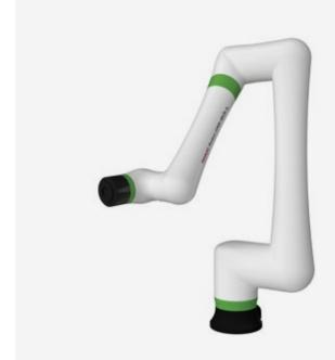
Collaborative robot that thanks to its reduced weight, can be easily installed in a wide range of applications, such as automated guided vehicles (AGVs). The robot can perform tipping movements highly functional in different applications.
