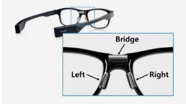
Electrooculographs Jins memes ES\_R are glasses that integrate three sensors (accelerometer, gyroscope and 3-point electrooculographic sensor) able to provide in output the electrooculogram (EOG), which is based on the potential difference existing between the cornea and retina. Through the EOG, stress and visual fatigue can be assessed.
